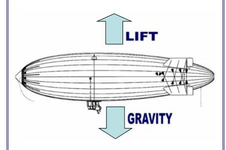
The static lift generated as a result of Archimedes principle, and the force of gravity are precisely balanced
