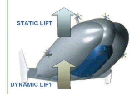
Dynamic lift is generated by its lifting body envelope. The principle is the same as an aircraft wing with airspeed being required.
