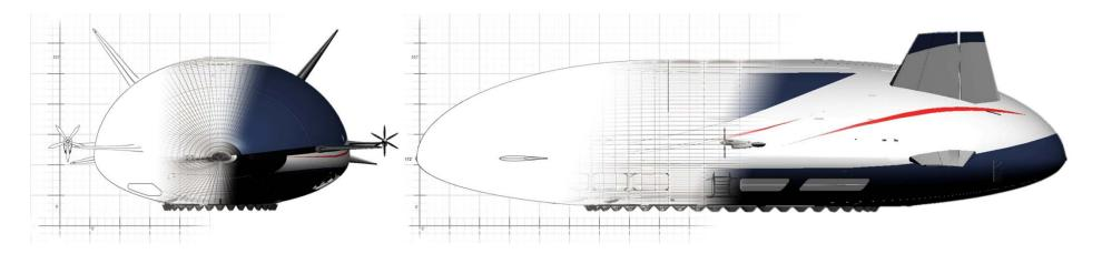
The Aeroscraft is a new type of rigid variable buoyancy air vehicle designed to control lift in all stages of air or ground operations including the ability to offload payload without re-ballasting. The key features of the Aeroscraft include the rigid structure, buoyancy management system, vertical takeoff and landing capabilities, and the ability to operate at low speed, in hover and from unprepared surfaces.
