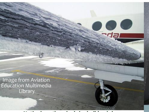
Notice how the wing's ice buildup is less on the leading edge's expandible rubber boot which had been employed prior to landing.
